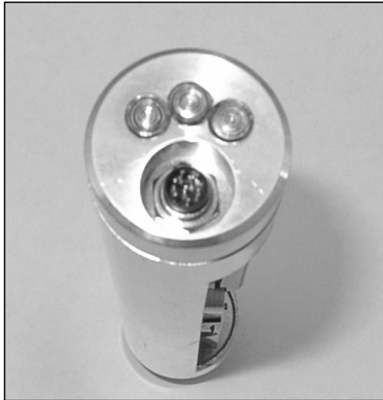
Figure 2.—MIDAS LED lights and serial connector
