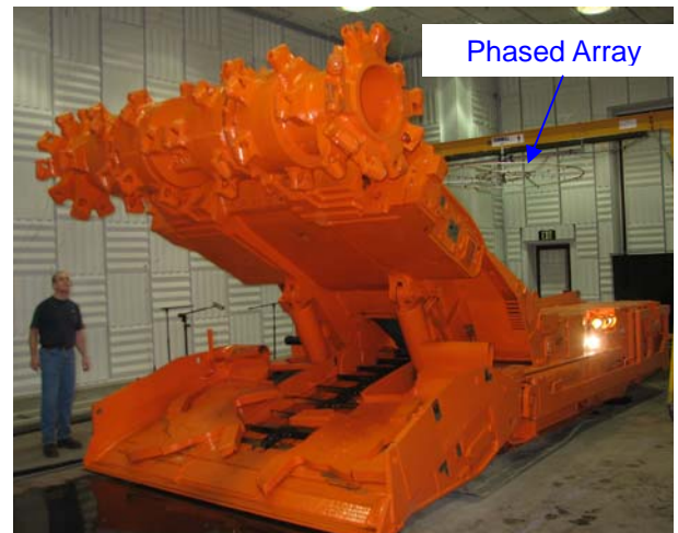
Figure 3. Continuous Miner in the Hemi-Anechoic chamber.
