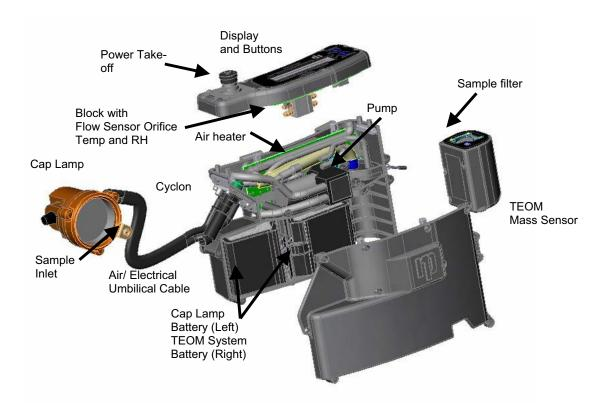
Figure 2. PDM internal components.
