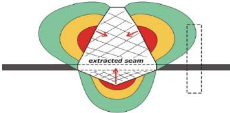
Figure 3. A generalized roof control mechanism defined by movement of ground within the pressure arch surrounding the mine opening. (Courtesy of SCT Operations, Australia).
