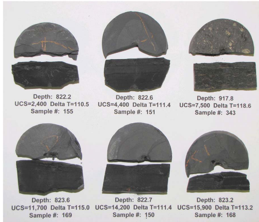
Fig. 13. Carbonaceous shale samples from corehole Kentucky A. The samples have been tested and the halves oriented to show a top view and a view of the failure surface. All samples are from the Anna shale, except the top right sample, which is from the Turner Mine shale. The samples were chosen to illustrate the wide range of UCS values observed in the carbonaceous shales, despite a narrow range of logged travel times. Depths in feet, UCS in psi and Delta T in \mu\text{s}/\text{ft} .
