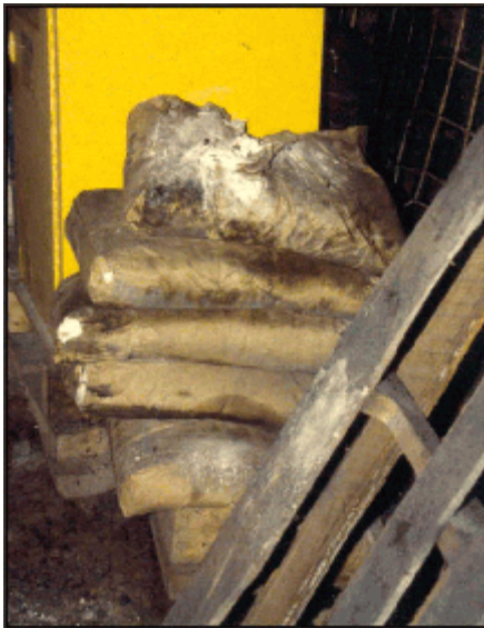
Figure 11.—Rock dust storage unprotected.
