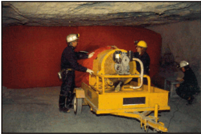
Figure 7.—Inflatable feed-tube partition in the Lake Lynn Experimental Mine.
