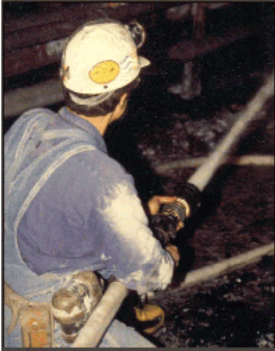
Figure 2.—Measuring the throw distance of water hose.
