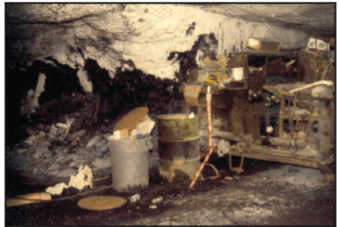
Figure 16.—Improper storage of underground trash.
