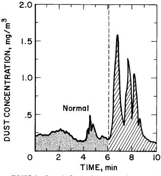
FIGURE 5.—Case 3: Operator's exposure from blowing clothes with compressed air.
