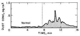
FIGURE 10.—Case 9: Operator's exposure from coworker sweeping floor one level down.
