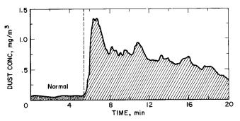
FIGURE 9.—Case 8: Operator's exposure from bag hopper overflowing.
