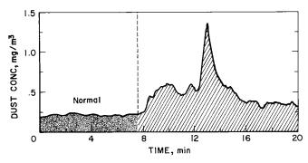
FIGURE 8.—Case 7: Operator's exposure from bulk loading outside.
