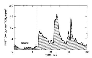
FIGURE 7.—Case 6: Operator's exposure from broken bag during conveying process.
