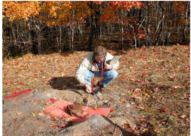
Figure 2. Borehole monitoring with sampling wand.
