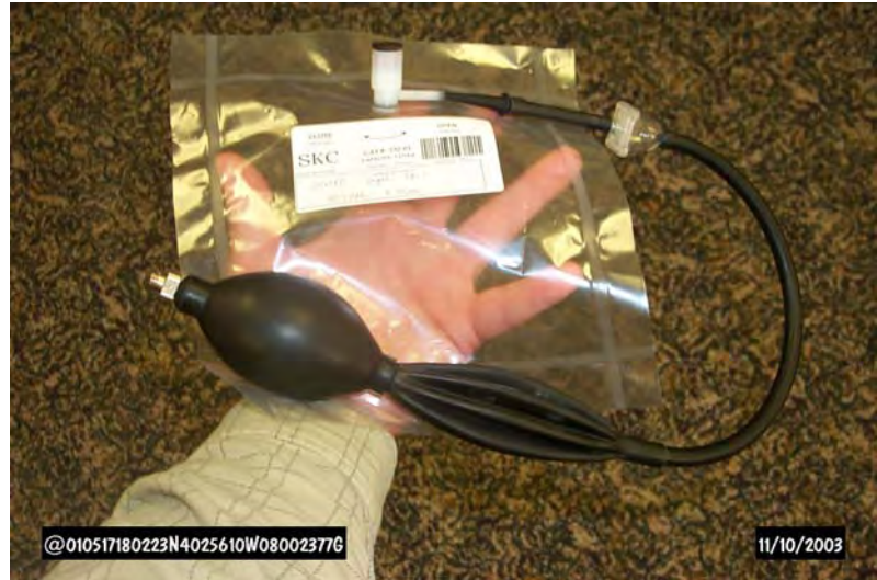
Figure 4. Aspirator pump and Tedlar bag.
