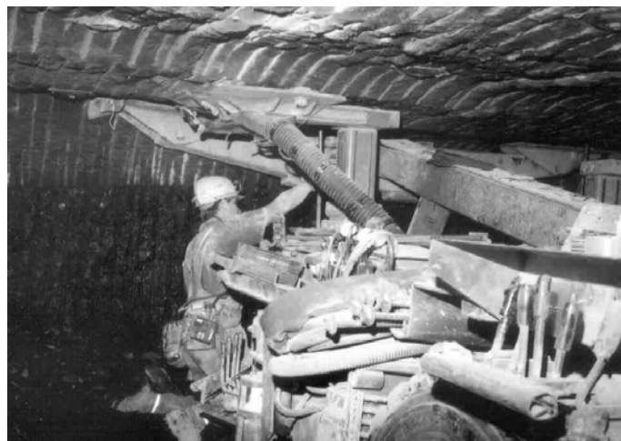
Figure 4. Canopy air curtain installed on roof bolter.
