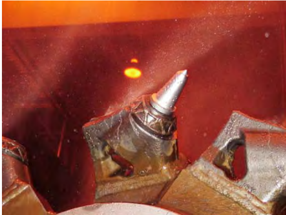
Figure 1a. Wet head bit block showing water spray behind the bit.
