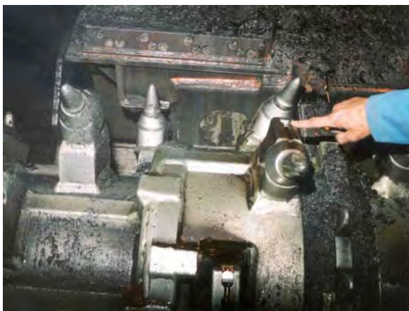
Figure 1b. Wet head sprays on continuous miner cutter head.
