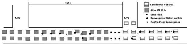
Figure 5. Tailgate test site with the location and type of the cribs and instrument location being noted. The sand props were not part of the study.
