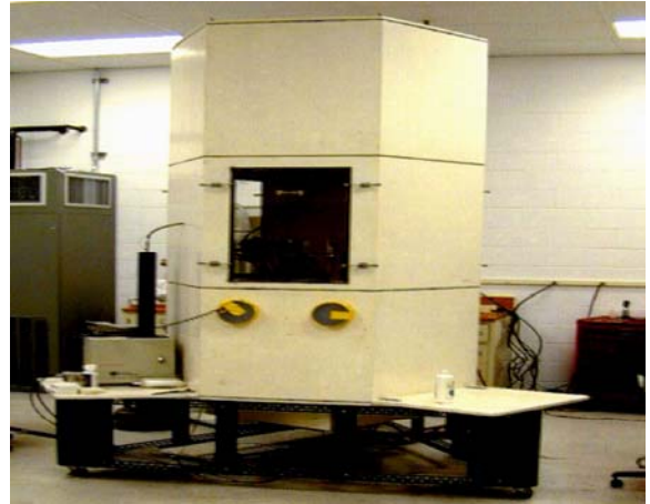
Figure 6. Schematic (A) and photograph (B) of the dust box where the response to diesel exhaust particles was measured.
