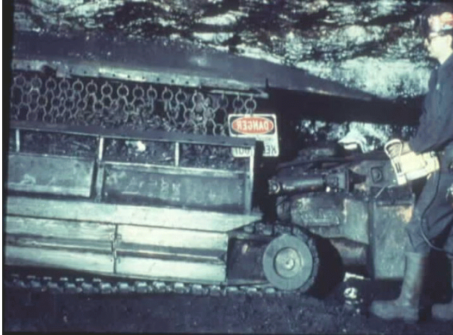
Figure 8. A Mobile Roof Support (MRS).
