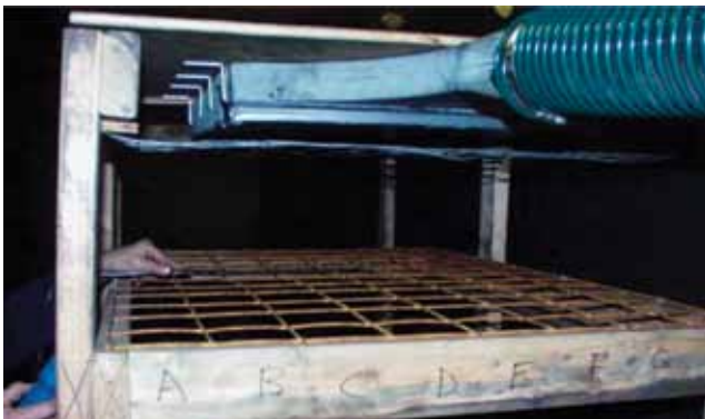
Velocity measurement grid 25.4 cm (10 in.) beneath the plenum.
