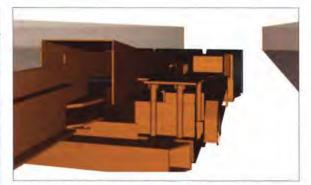
Figure 5: Operator's eye view, which allows the researchers to analyze the positions that the miner takes trying to see VALs while operating the machine.
