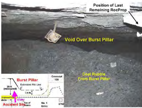
Figure 7. 20-ft deep void over pillar on right side of No. 1 entry following August 16 accident (After Gates et al., 2008).
