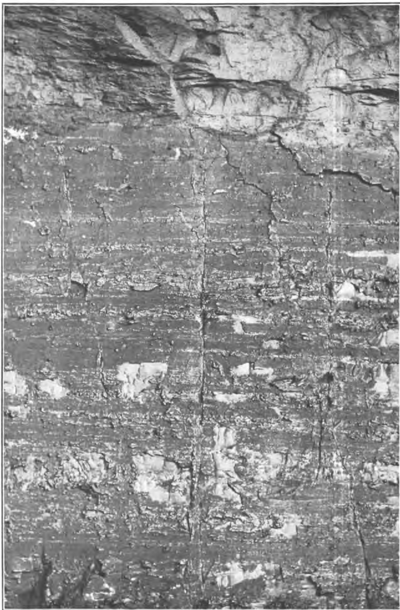
COKE BUBBLES FORMED ALONG BEDDING PLANES OF COAL TEST 2.
