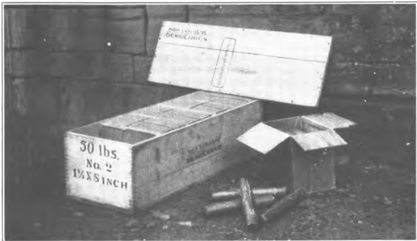
B. BOXES OF DYNAMITE, SHOWING METHOD OF PACKING IT.
