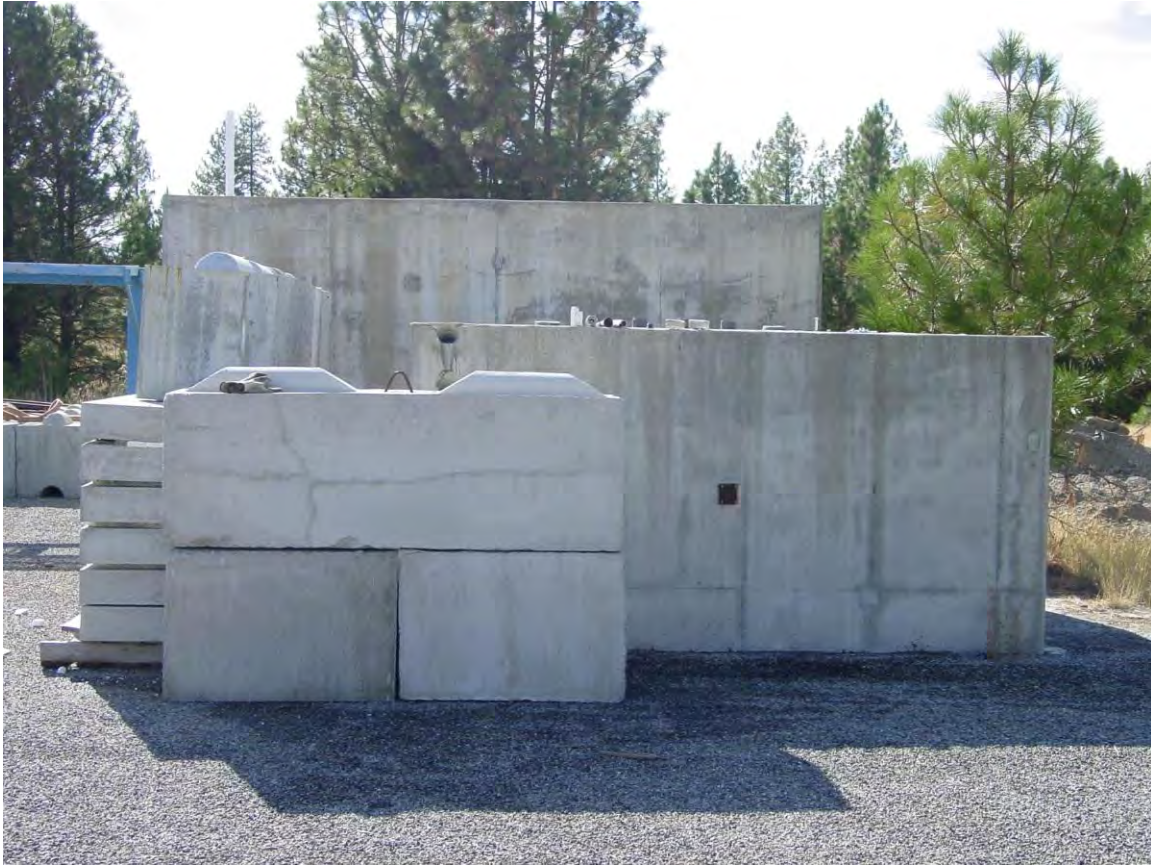
Fig. 2. Photograph of block experiment prior to test showing placement of barrier blocks to restrain fly rock.
