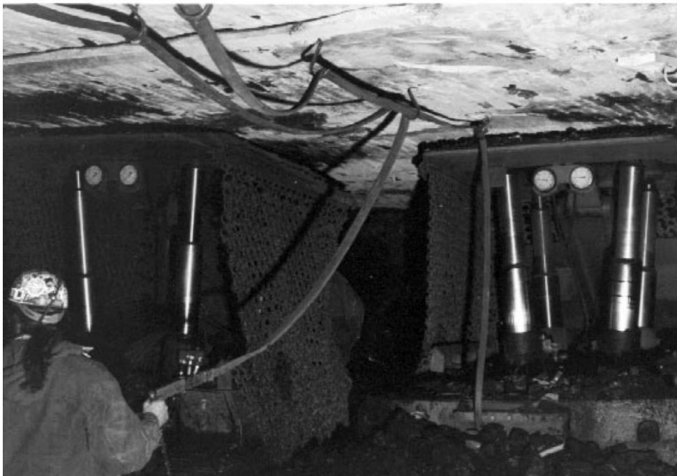
Figure 3.—Full pillar extraction using mobile roof supports.
