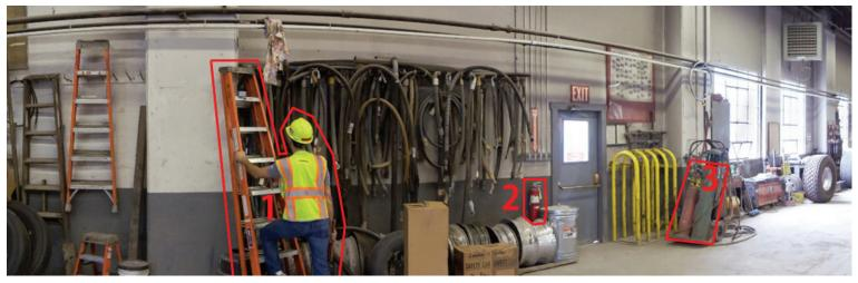
Figure 2: Example of three hazards outlined in red from EXAMiner, taken from the left side of the panoramic image of the shop shown in Figure 1.
