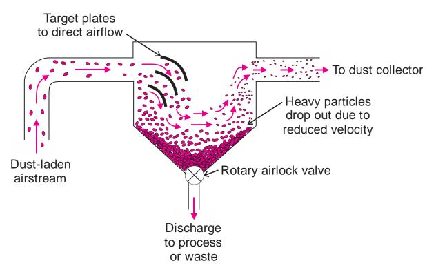
Figure 2.15. Illustration showing a typical design of a gravity separator (drop-out box).
