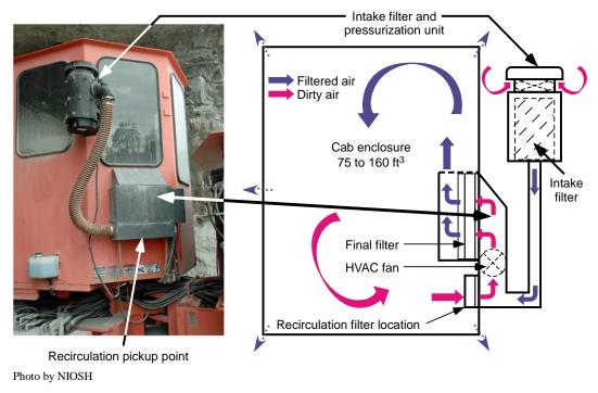
Figure 10.3. Intake, recirculation, and final filter locations within an HVAC system designed by an original equipment manufacturer and field tested by NIOSH.
