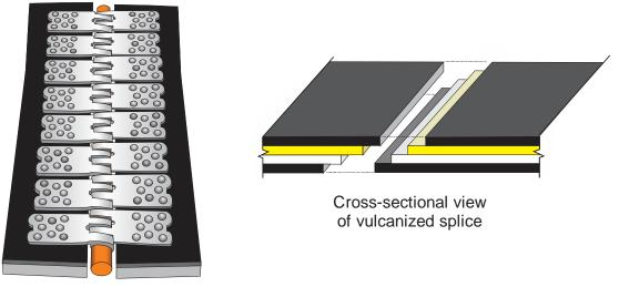
Figure 6.21. Illustration of a mechanical belt splice (left) and a vulcanized belt splice (right).
