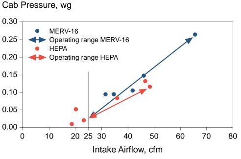
Figure 10.14. Graphical comparison of the intake airflows and positive cab pressures for a face drill test at a mine site comparing MERV-16 and HEPA filters.
