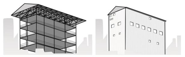
Figure 9.12. Illustration of an open structure design compared to a standard walled structure.
