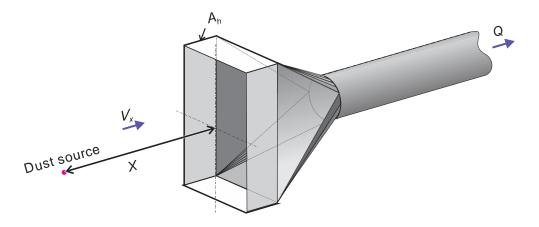
Figure 2.7. Illustration demonstrating the use of a hood entry loss calculation to determine the exhaust volume needed for a basic freestanding hood arrangement [adapted from ACGIH 2010].
