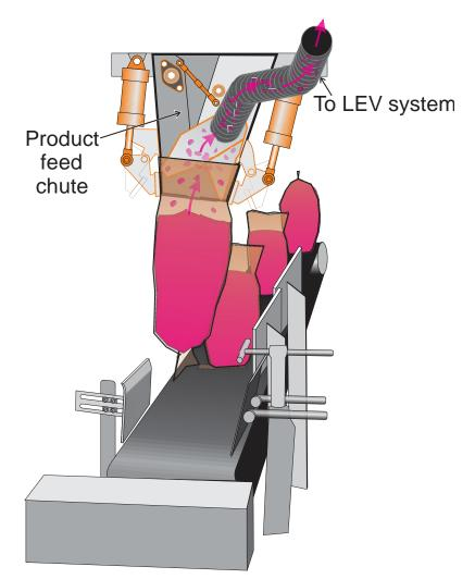
Figure 7.5. Illustration showing an open-top bag being loaded with product. The product is normally whole grain material, which is less dusty.
