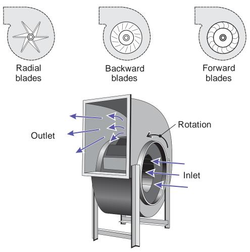
Figure 2.31. Illustration of a typical centrifugal fan.
