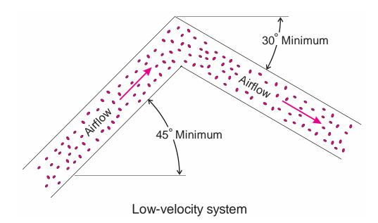
Figure 2.12. Illustration of duct design angles for low-velocity systems.
