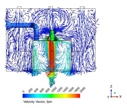
Figure 4.11. Velocity vectors for a cross-sectional plane (shroud without air-blocking shelves) with a detailed view underneath the table.
