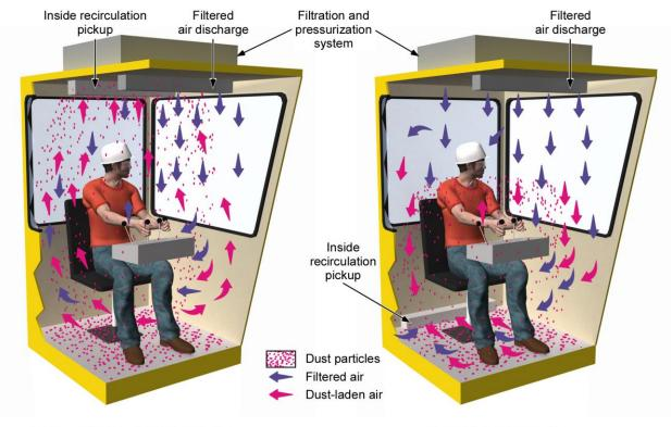
Intake and return at roof flow design
