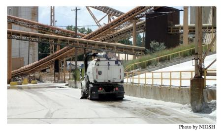
Figure 9.18. Sweep truck cleaning an outside roadway, typically used at plants and mills.
