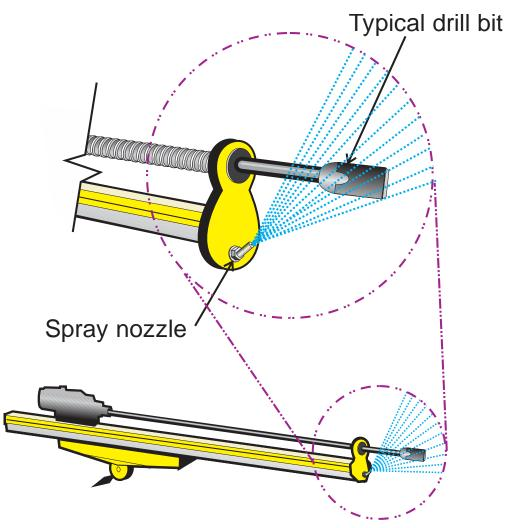
Figure 4.21. Illustration of drill boom showing external water sprays directed onto the drill steel and toward the collar of the hole.
