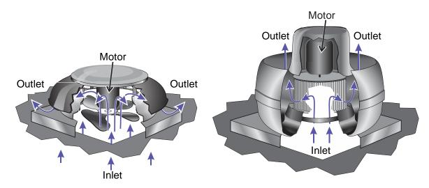
Figure 2.33. Illustration of typical roof ventilators using axial fans (left) and centrifugal fans (right).
