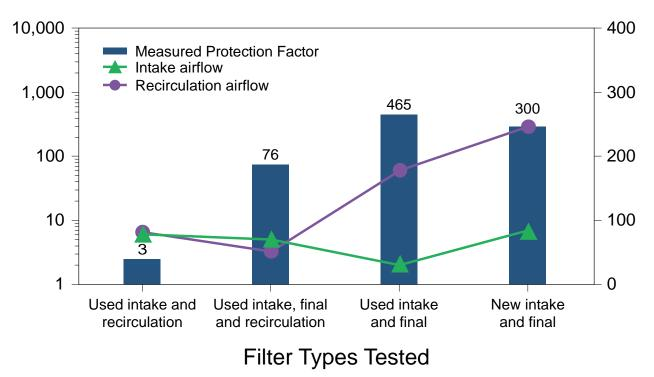
Figure 10.5. Bar chart comparison of cab performance variations with respect to different filters used in a filtration and pressurization system in a field study.
