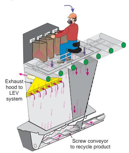
Figure 7.9. Illustration of an exhaust hopper below a bag loading station with an integrated LEV system to capture dust generated during the bag loading process.
