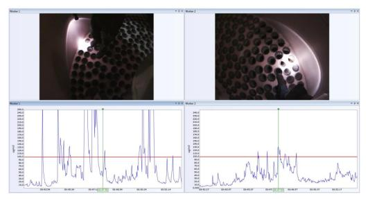
Figure 9.1. Screenshot from the EVADE software showing video stills and respirable dust exposures for two coworkers. The video stills and graphs show respirable dust exposures for Worker 1 (left) and Worker 2 (right) while changing filter canisters inside the same local exhaust ventilation system at the same time (i.e., in the same confined space). Note that the respirable dust exposure of Worker 1, who was wearing a contaminated sweatshirt, was three times higher than that of Worker 2.
