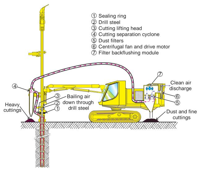
Figure 4.18. Illustration of a typical dust collector system used by small crawler (or "buggy") drills.
