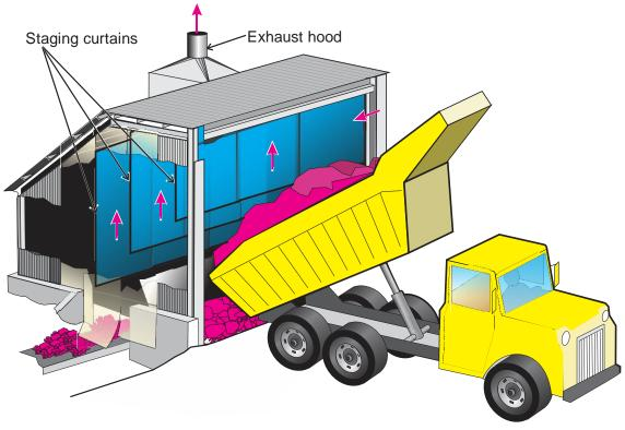
Figure 5.5. Illustration of a dry (exhaust) dust control system with a partial enclosure at a crusher dump loading operation.
