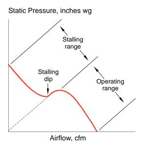
Figure 2.28. Graph of a fan performance curve showing stalling and operating ranges.
