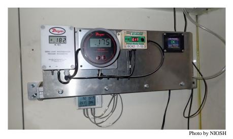
Figure 10.16. Comparison test of three pressure monitors at a crusher booth at an underground mine compared to a certified pressure reference instrument. The Dwyer gauge is on the far left.
