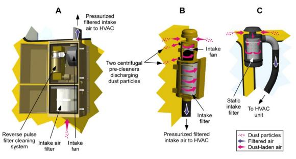
Figure 10.8. Illustration of two types of recommended powered intake systems. A and B show a powered unit design (recommended) while C shows a static, non-powered system (not recommended).
