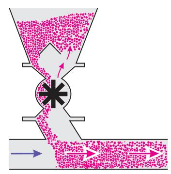
Figure 6.27. Illustration of a rotary airlock feeding a pneumatic conveying line.
