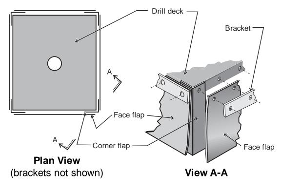
Figure 4.5. Illustration of reinforcing flaps added to each corner of a rectangular deck shroud to reduce leakage.
