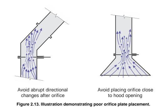
Orifice plates should also not be installed near hood inlet openings. The higher velocities near the orifice tend to capture unwanted material. Hood capture velocities below 500 fpm should be maintained. On fine-grind materials, a target capture velocity of 200 fpm is desirable.
