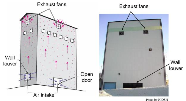
Figure 9.11. Illustration and photo showing the basic design of a total structure ventilation system.
