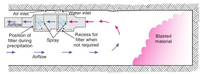
Figure 4.25. Illustration of a filtration unit, located in the blast heading, used for filtering contaminated ventilation air from the blast heading after blasting occurs.
