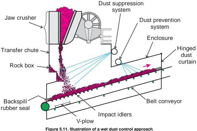
on a crusher discharge/belt loading operation.
