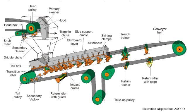
Figure 6.1. Illustration of the basic components of a conveyor belt.
