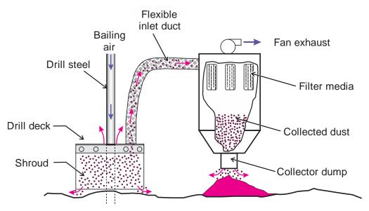
Figure 4.4. Illustration of a basic dry dust collector system on a drill.
