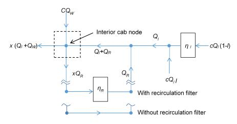
Figure 10.2. Two- and one-filter cab systems with and without a recirculation filter. Q's denote air quantities, x's & c's denote contaminant concentrations, and η's denote filter efficiencies.
