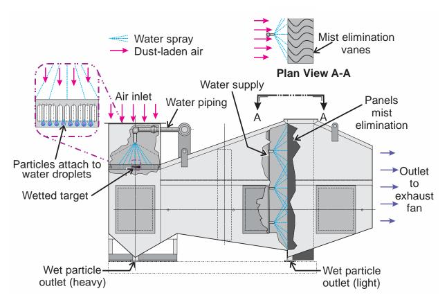
Figure 2.22. Illustration showing a typical design of a wet scrubber dust collector.
