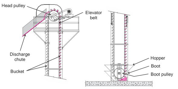
Figure 6.23. Illustration of a bucket elevator.
