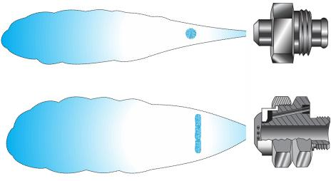
Figure 3.6. Two types of nozzle spray patterns. The top illustration shows a typical air atomizing nozzle round spray pattern. The bottom illustration shows a typical fan spray pattern [adapted from SSCO 2018].
