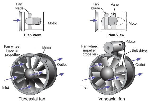
Figure 2.30. Illustration of a typical tubeaxial fan (left) and vaneaxial fan (right).
