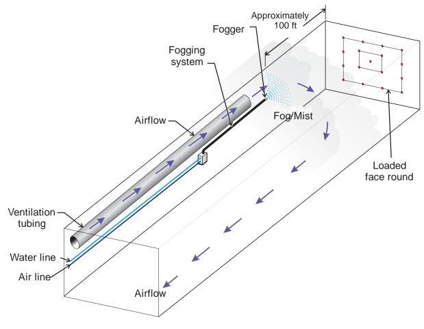
Figure 4.23. Illustration of a fogger spray used to create a mist for dust suppression in the heading where blasting will occur.
