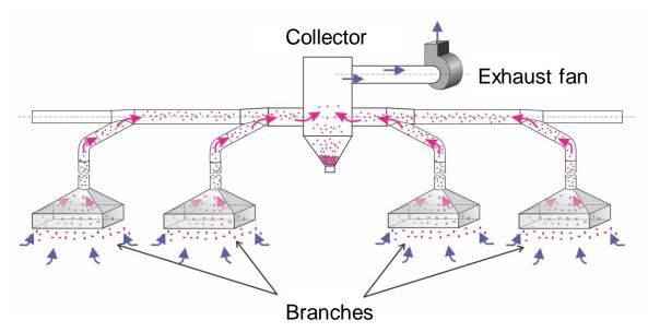
Figure 2.26. Illustration of how a complex exhaust system is a combination of branches linking simple exhaust systems [adapted from ACGIH 2010].
