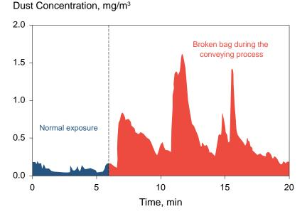
Figure 9.23. Graph showing the increase in a worker's respirable dust exposure from a broken bag during the conveying process.
