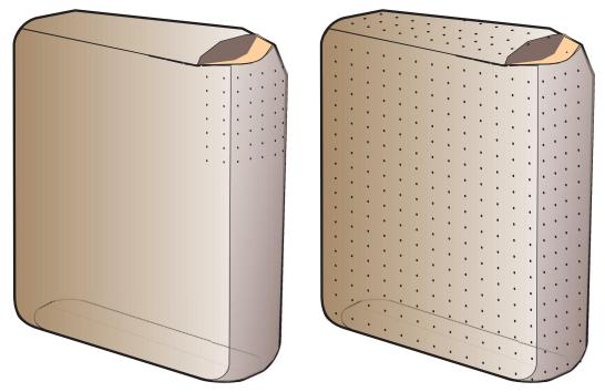
Figure 7.3. Two types of bag perforations. The left illustration shows undervalve perforations. The right illustration shows overall perforations.
