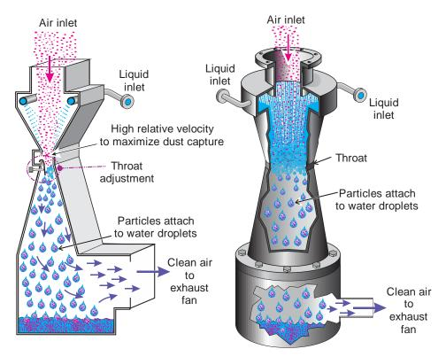
Figure 2.23. Illustration of typical designs for a venturi scrubber.
