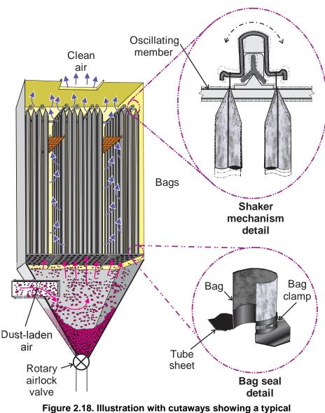
design of a mechanical shaker dust collector.
