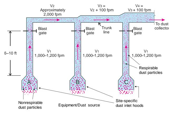
Figure 2.14. Illustration of the horizontal ( $V_{2,3,4}$ ) and vertical ( $V_1$ ) velocity relationship in a modified low-velocity system. Nonrespirable (larger) dust particles fall back into the process, while respirable (smaller) particles are transported through the ductwork to the dust collector.
