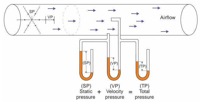
Figure 2.1. Illustration of the relationship between static pressure, velocity pressure, and total pressure [adapted from ACGIH 2010]. Example represents suction side of the fan.
