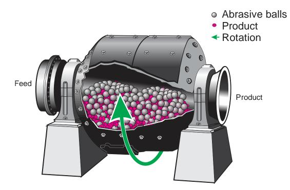
Figure 5.12. Cutaway illustration of a ball mill.
