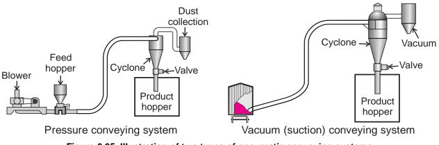
Figure 6.25. Illustration of two types of pneumatic conveying systems.
