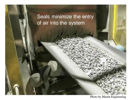
Figure 6.14. Demonstration of material being transported into a sealed head chute.
