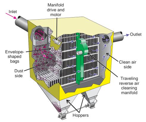
Figure 2.19. Illustration showing a typical design of a reverse air dust collector.
