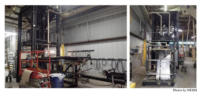
Figure 7.15. FFS system in service loading larger-grain play sands.
