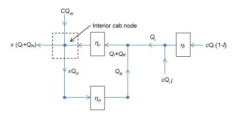
Figure 10.4. Three-filter cab system with the final filter downstream of the intake and recirculation filters. Q's denote air quantities, x's & c's denote contaminant concentrations, and  $\eta$ 's denote filter efficiencies.
