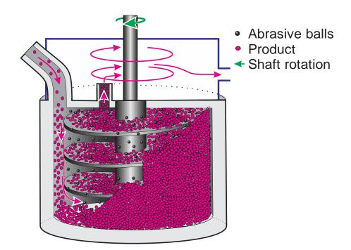
Figure 5.13. Cutaway illustration of a stirring mill.
