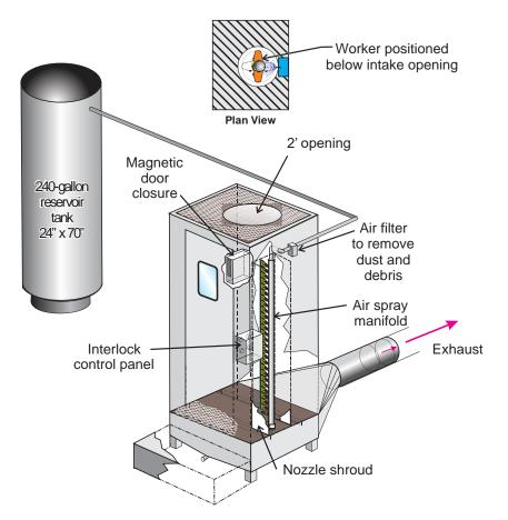
Figure 9.2. Illustration of the overall design of a clothes cleaning system.
