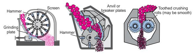
Figure 5.3. Illustrations of three examples of impactive crushers. The left illustration shows a hammermill crusher with material being crushed between the rotating hammers and a fixed grinding plate. The center illustration shows material being crushed between rotating hammers and fixed anvil plates in an impact breaker. The right illustration demonstrates the size-reduction action of a toothed roll crusher.
