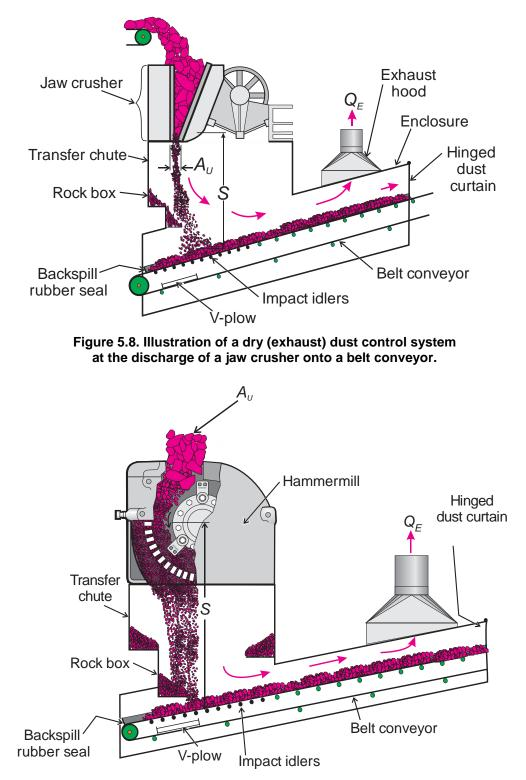
Figure 5.9. Illustration of a dry (exhaust) dust control system at the discharge of a hammermill crusher onto a belt conveyor.
