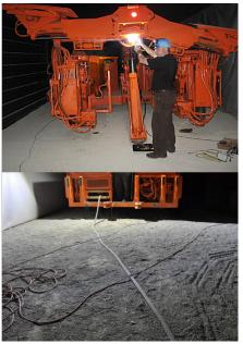
Figure 2: The existing illumination provided by traditional lighting for a roof bolter (left). The improved illumination provided by the NIOSH-developed Saturn LED area light (right).
