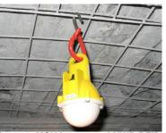
Figure 3. MSHA-approved UWB RFID tag with an estimated 10-year battery life.
