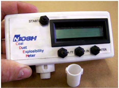
Figure 41. Coal Dust Explosibility Meter.
