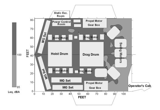
Figure D–9.—Leq<sub>(A)</sub> sound levels in house of Marion 8750 dragline, 132-yd<sup>3</sup> bucket.
