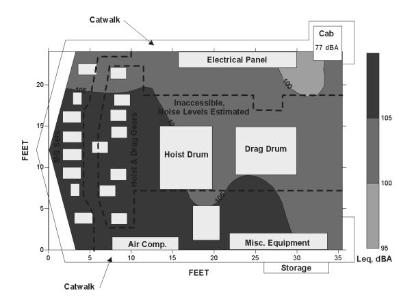
Figure D–6.—Leq<sub>(A)</sub> sound levels in house of Marion 195M dragline.
