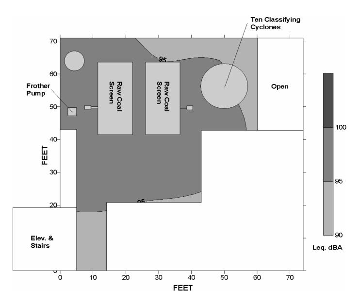
Figure F–4.—Leq<sub>(A)</sub> sound levels on a floor with only two vibrating screens.
