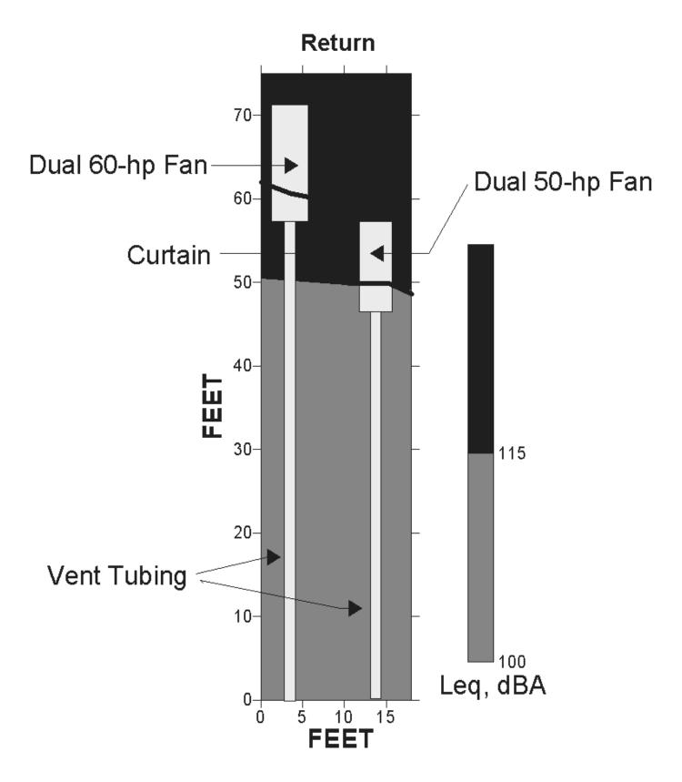
Figure B–9.—Leq<sub>(A)</sub> sound levels around Spendrup Dual 50 and Dual 60 hp fans.
