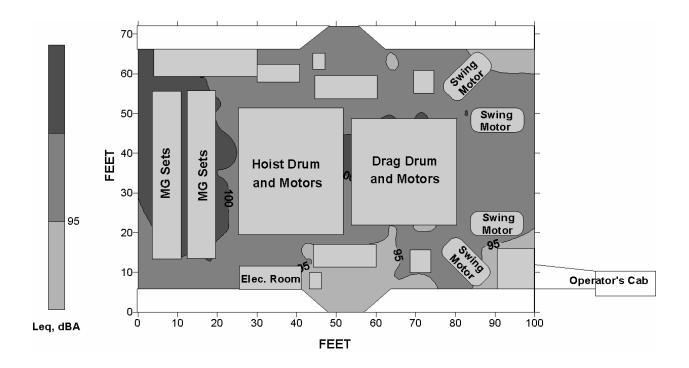
Figure D–2.—Leq<sub>(A)</sub> sound levels in house of Page 757 dragline.
