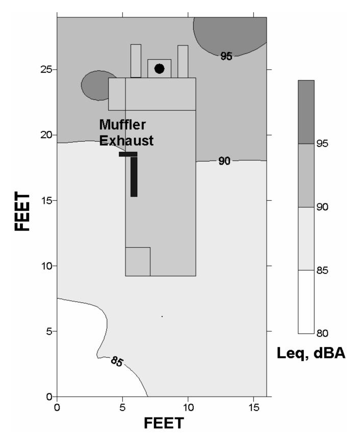
Figure B–6.—Leq<sub>(A)</sub> sound levels around a Fletcher Model DR–15–E single-boom roof bolting machine.
