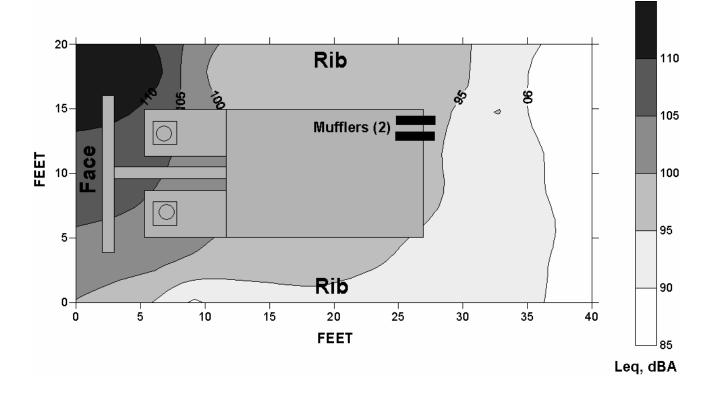
Figure 10.—Sound profile of sound levels around a dual-boom roof bolter.
