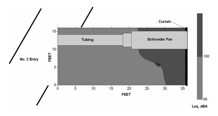
Figure 11.—Leq<sub>(A)</sub> sound levels around a Schroeder Model 271 auxiliary fan.
