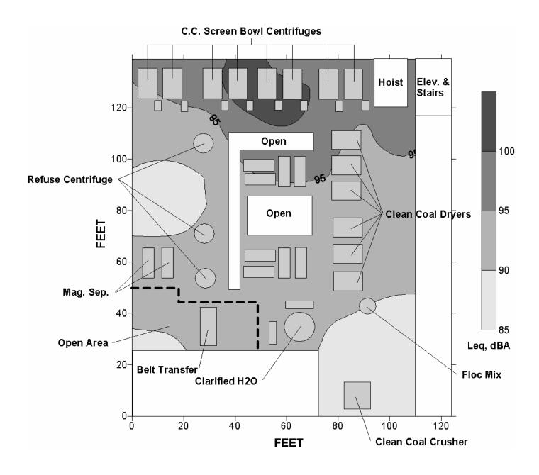
Figure 29.—Example of a variable-sound-level preparation plant floor.
