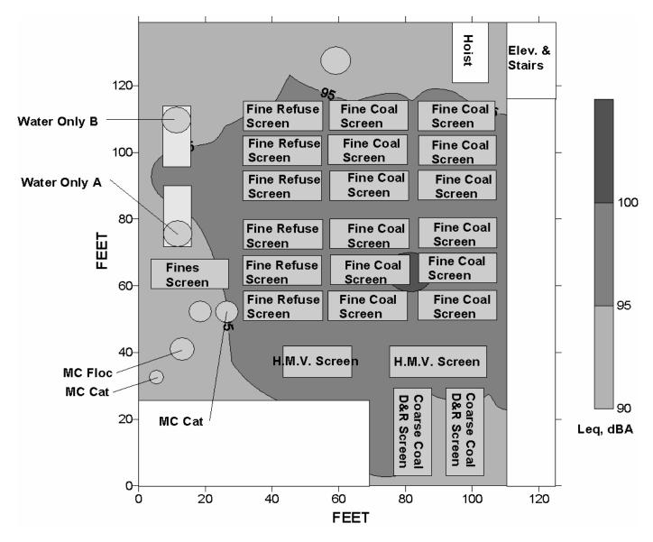
Figure F–1.—Leq<sub>(A)</sub> sound levels on a floor with many (23) vibrating screens.
