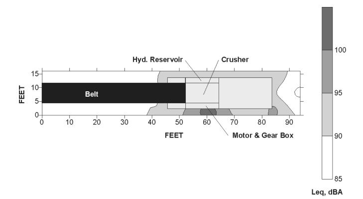
Figure B–7.—Leq<sub>(A)</sub> sound levels around a McLanahan HV–50 feeder-breaker.
