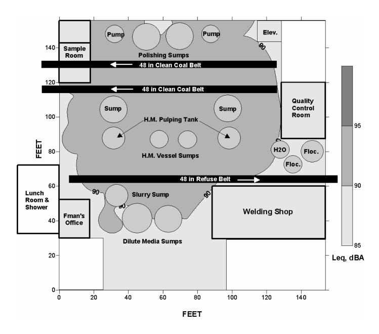
Figure F–6.—Leq<sub>(A)</sub> sound levels on bottom floor containing sumps, pumps, and belts.
