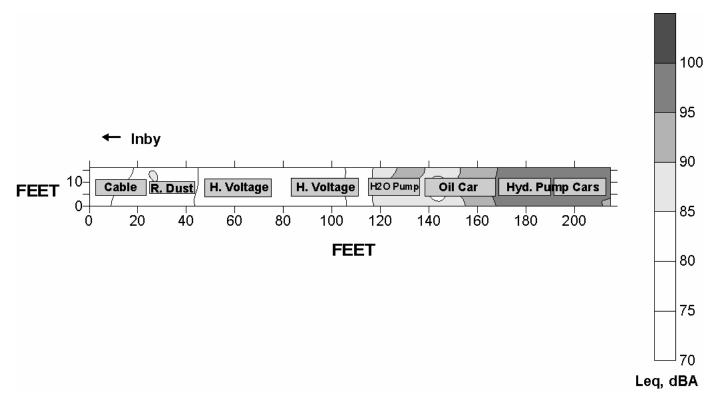
Figure B–12.—Leq<sub>(A)</sub> sound levels around longwall hydraulics.
