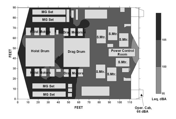
Figure D–10.—Leq<sub>(A)</sub> sound levels in house of Marion 8750 dragline, 110-yd<sup>3</sup> bucket.
