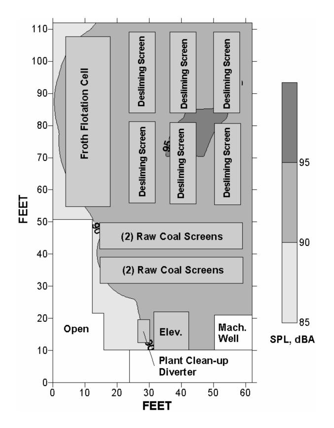
Figure F–3.—Leq<sub>(A)</sub> sound levels on a floor with eight vibrating screens.
