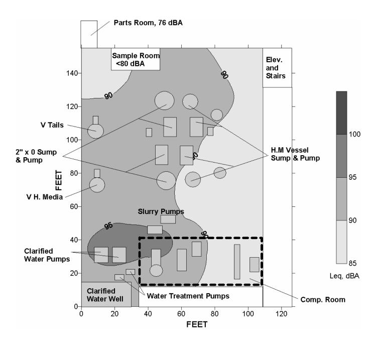
Figure F–5.—Leq<sub>(A)</sub> sound levels on bottom floor containing sumps and pumps.
