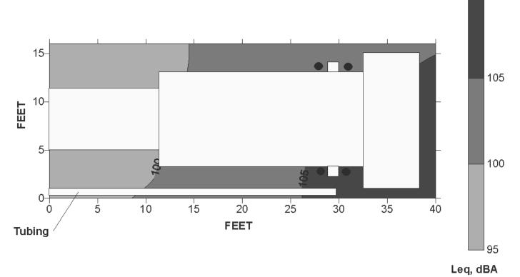
Figure B–4.—Leq<sub>(A)</sub> sound levels around an Alpine miner/bolter during mining and bolting.
