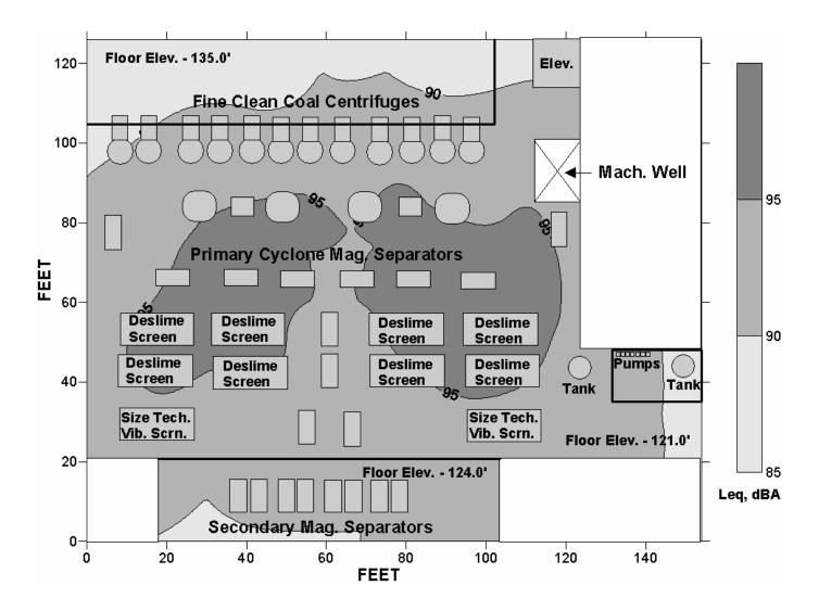
Figure F–12.—Leq<sub>(A)</sub> sound levels on floor with various types of processing equipment.
