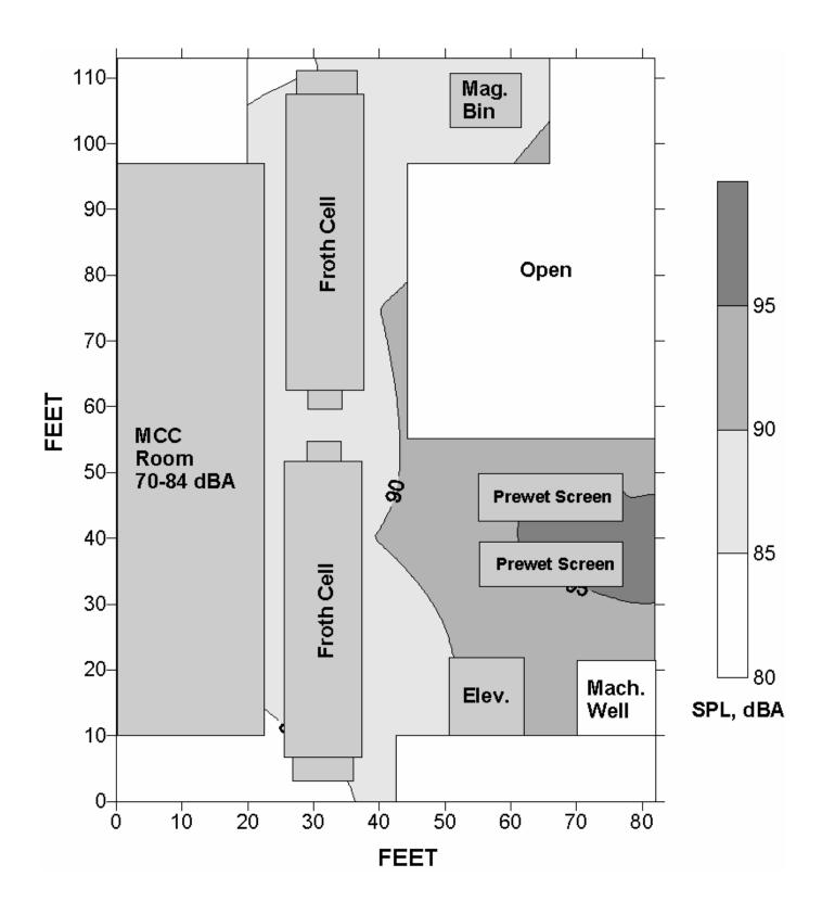
Figure F–10.—Leq<sub>(A)</sub> sound levels around froth flotation cells.
