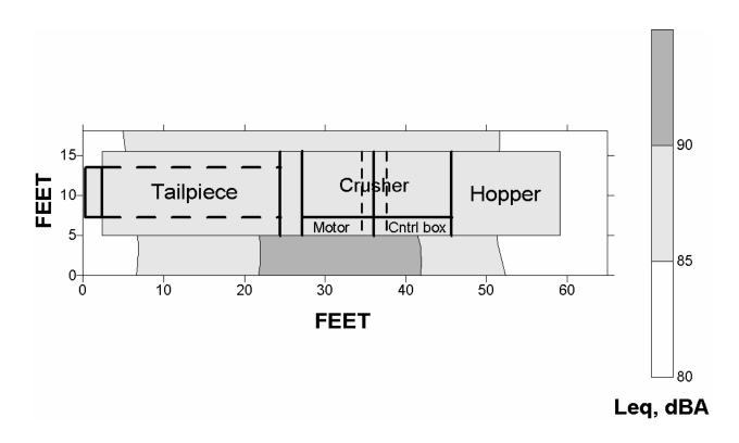
Figure B–8.—Leq<sub>(A)</sub> sound levels around a Stamler Model BF–14A–1Z–530 feeder-breaker.
