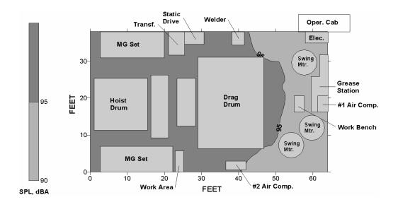
Figure D–7.—Leq<sub>(A)</sub> sound levels in house of Marion 7800 dragline.
