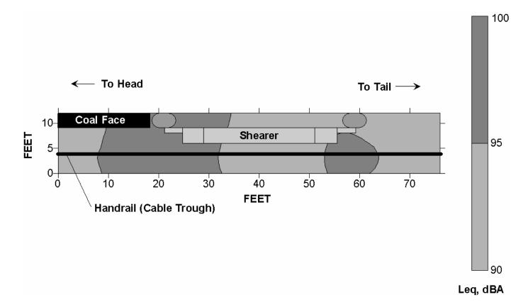
Figure B–10.—Leq<sub>(A)</sub> sound levels near shearer while cutting from tail to head.
