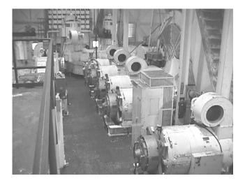
Figure 16.—Example of hoist and/or drag motors.
