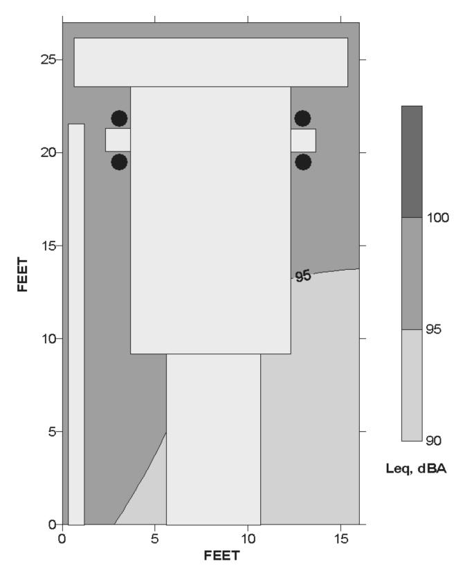
Figure B–2.—Leq<sub>(A)</sub> sound levels around a Joy miner/bolter during bolting cycle.
