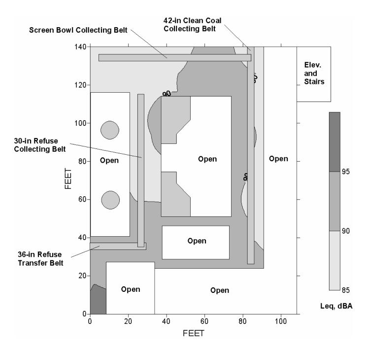
Figure F–11.—Leq<sub>(A)</sub> sound levels on floor with primarily belts.
