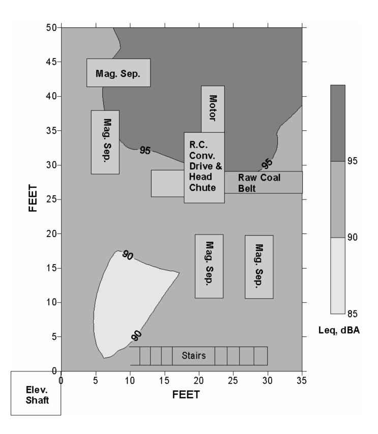
Figure F–7.—Leq<sub>(A)</sub> sound levels on top floor containing raw coal feed belt.
