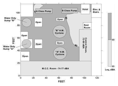
Figure 27.—Example of a low-sound-level preparation plant floor.
