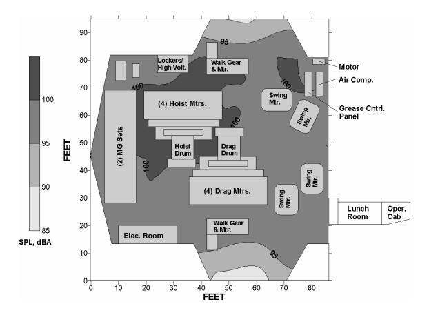
Figure D–8.—Leq<sub>(A)</sub> sound levels in house of Marion 8200 dragline.
