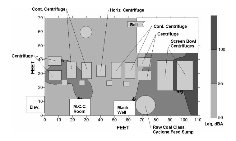
Figure F–8.—Leq<sub>(A)</sub> sound levels on floor with mostly centrifuges.
