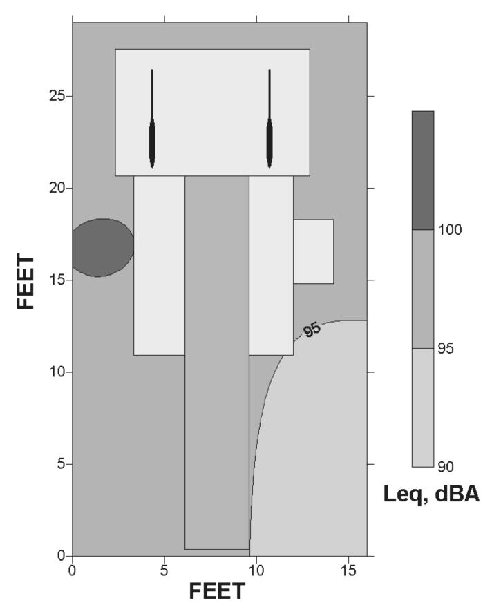
Figure B–5.—Leq $_{(A)}$  sound levels around a Joy Model 14BU10 loading machine.
