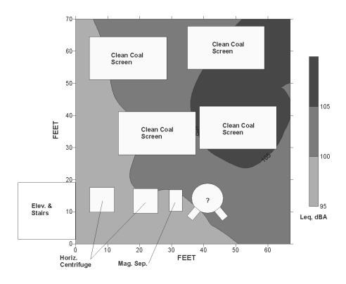
Figure 28.—Example of a high-sound-level preparation plant floor.
