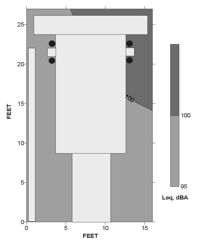
Figure B–1.—Leq<sub>(A)</sub> sound levels around a Joy miner/bolter during mining.
