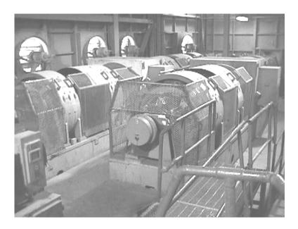
Figure 15.—Motor-generator sets in back of dragline.
