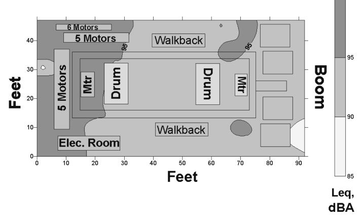
Figure D-1.—Leq<sub>(A)</sub> sound levels in house of Page 752 dragline [Bauer and Babich 2003, 2004b].
