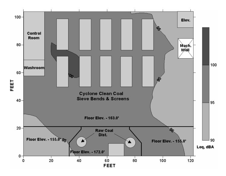
Figure F–2.—Leq<sub>(A)</sub> sound levels on a floor with 10 vibrating screens.
