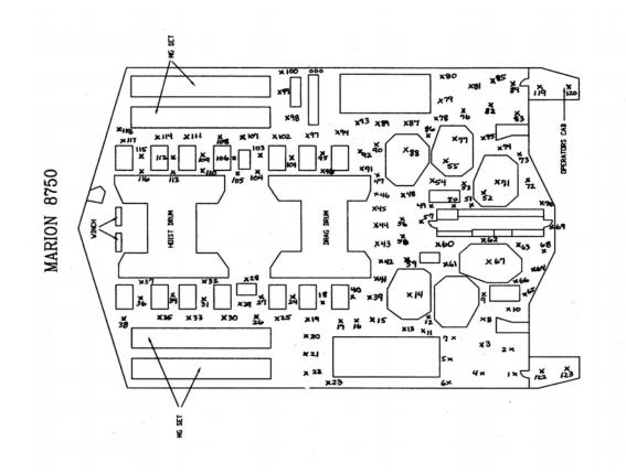
Figure 14.—Example of sound level measurement locations (x15) in a dragline.
