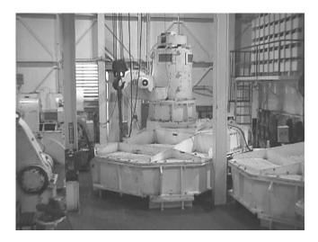
Figure 17.—Swing motor and gear.
