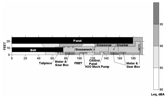
Figure B–11.—Leq<sub>(A)</sub> sound levels around a longwall stageloader.
