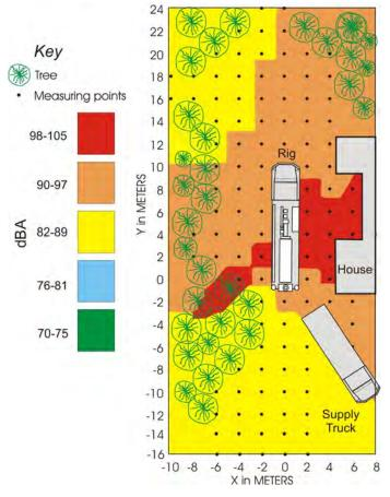
The drill rig's compressor, engine, cooling fan, and drill rod are noise sources that can expose workers to noise levels 90 dB(A) and above.
