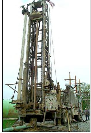
Be sure that winch and hoist cables will remain at least 10 feet from power lines during all drilling and well maintenance operations.
