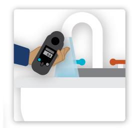
3. Jason increases the frequency of measuring chlorine levels at the taps from weekly to daily to ensure that adequate residual disinfectant is moving through the system.
