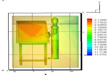
Figure 7 ATTILA model geometry and flux contours.
