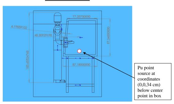
Figure A1 Dimensions (all lengths are in centimeters)
