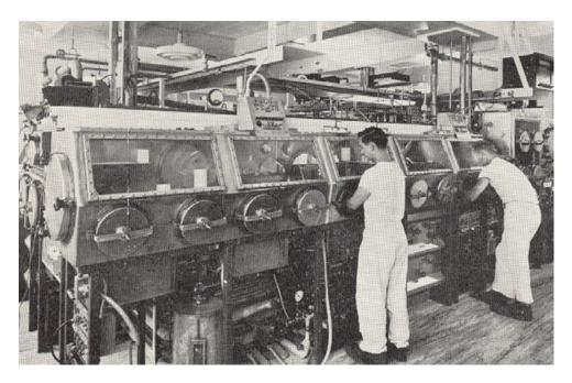
Figure 1 Plutonium gloveboxes at LANL  $^{(1)}$
