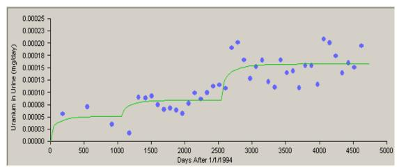
Figure A-8. Predicted values (line) versus measured results (blue dots), 1/1/1994 to 12/31/2006, 84th percentile, type M.
