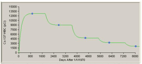
Figure B-122. Predicted cesium bioassay results calculated using IMBA-derived cesium intake rates (line) compared with bioassay results (dots) from all intakes, 50th percentile, type F.
