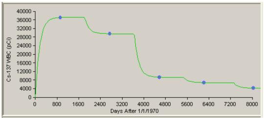
Figure B-123. Predicted cesium bioassay results calculated using IMBA-derived cesium intake rates (line) compared with bioassay results (dots) from all intakes, 84th percentile, type F.
