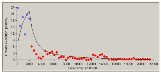
Figure B-113. Predicted uranium bioassay results calculated using IMBA-derived uranium intake rates (line) compared with bioassay results (dots), 1950 to 1955, 84th percentile, type S.
