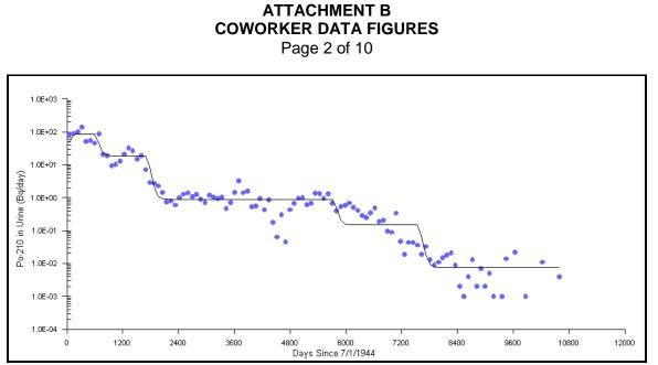
Figure B-3. Predicted (line) and observed (dots) 50th-percentile urinary excretion assuming inhalation intakes of type F <sup>210</sup>Po.
