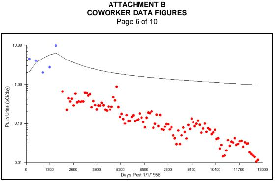
Figure B-11. Predicted (line) and observed (dots) 84th-percentile urinary excretion assuming inhalation intakes of type M plutonium, 1956 to 1960.
