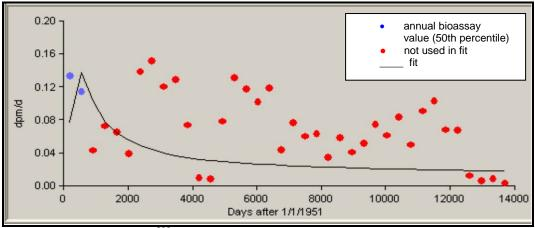
Figure A-18. Assumed <sup>239</sup>Pu intake, 1951 to 1952, 50th-percentile results, Type M.
