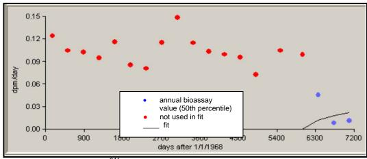
Figure A-25. Assumed <sup>241</sup>Am intake, 1985 to 1988, 50th-percentile results, Type M.
