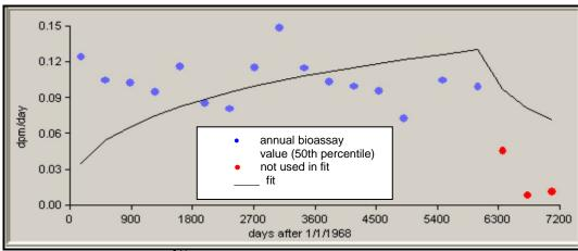
Figure A-24. Assumed <sup>241</sup>Am intake, 1968 to 1984, 50th-percentile results, Type M.
