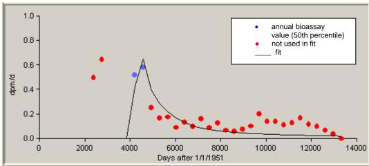
Figure A-14. Assumed <sup>234</sup>U intake, 1962 to 1963, 50th-percentile results, Type S.
