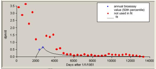
Figure A-12. Assumed <sup>234</sup>U intake, 1957 to 1958, 50th-percentile results, Type S.
