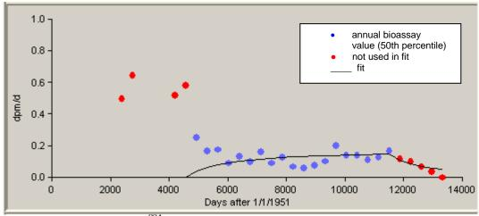
Figure A-15. Assumed <sup>234</sup>U intake, 1964 to 1982, 50th-percentile results, Type S.
