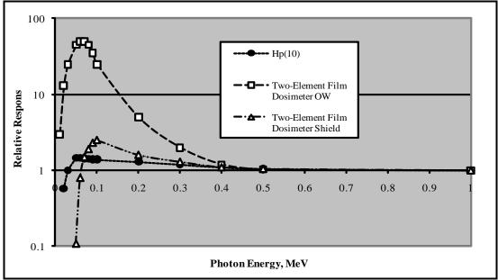
Figure 2-1. Measured two-element dosimeter photon response for anterior-to-posterior exposure geometry (Pardue et al 1944, Wilson et al 1990).
