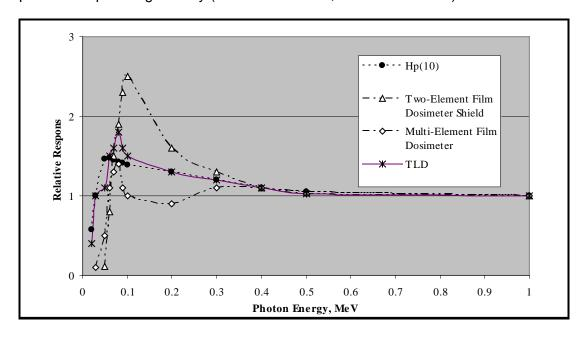
Figure 2-2. Measured deep dose response for Hanford Two-Element film, multielement film and thermoluminescent dosimeter compared to  $H_p(10)$ . (Wilson et al 1990).
