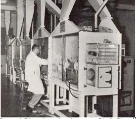
Figure 2 Plutonium gloveboxes at Chalk River<sup>(1)</sup>
