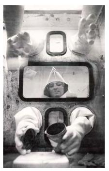
Figure 5 Other plutonium gloveboxes at Hanford. Note the viewing area in direct line with the lower torso in the center between the gloves. <sup>(2)</sup>
