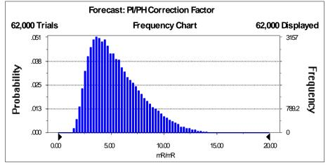
Figure 8 Intermediate and high energy photon correction factor distribution
