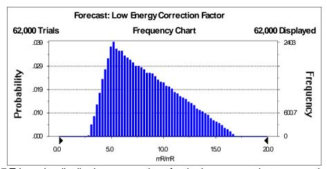
Figure 7 Triangular distribution assumptions for the low energy photon correction factor
