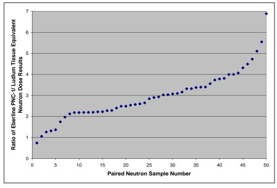
Figure 4: Ratio of Neutron Dose Rates (Eberline PNC-1 Neutron Detector/Ludlum Tissue Equivalent)
