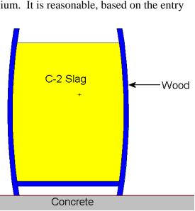
Figure A-2. Cross-Section of MCNP Model of Slag in a Whiskey Barrel
