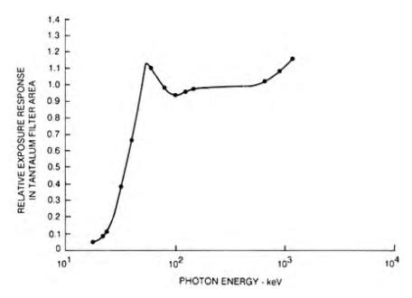
Figure 1. Film Response with 0.020-inch Tantalum Filter (adapted from Brady and Iverson, 1968) (Lalos 1989, Figure 2-5)
