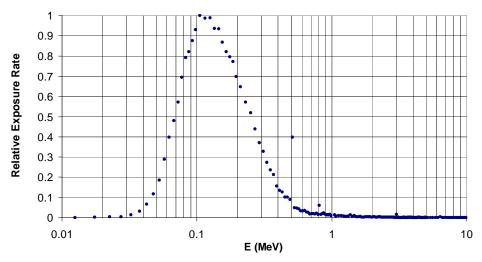
Figure 3. Exposure Rate vs. Photon Energy in Control Room (location #1 in Figure 2)
