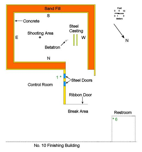
Figure 2. MCNP Model of New Betatron Building, Showing Locations of Exposure Assessments
