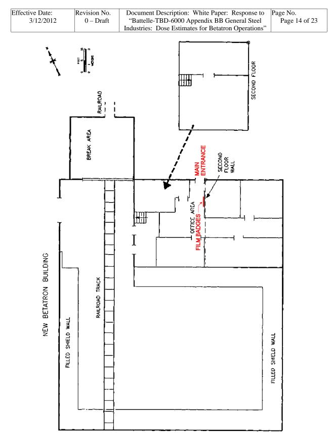
Figure 5. Floor Plan of New Betatron Building, Showing Location of Rack for Storing Film Badges. (Original drawing from Murray and Uziel 1992—entries in red by present authors)
