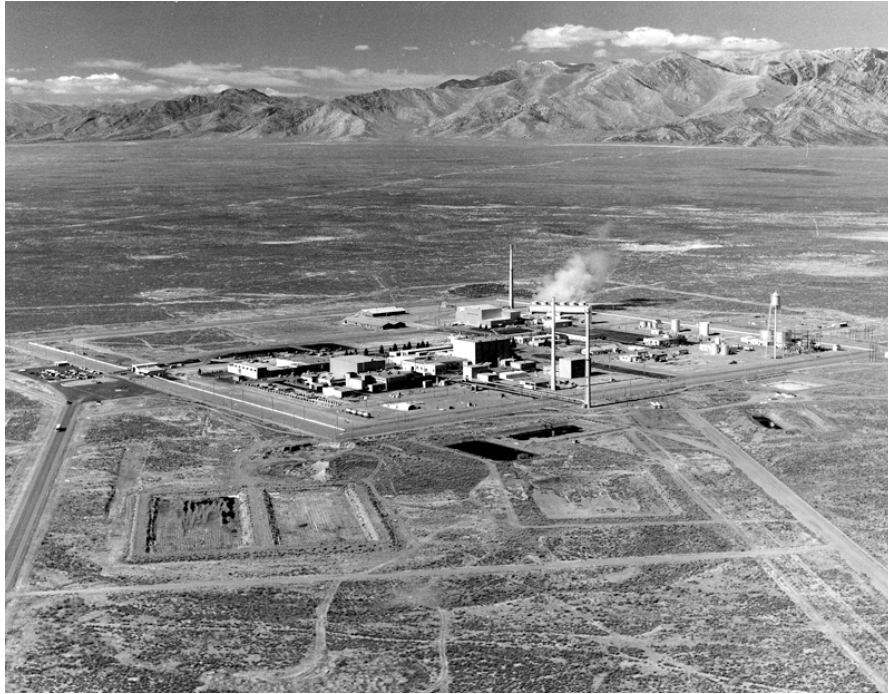
Figure 5. Test Reactor Area (TRA) at the INEEL where the Materials Testing Reactor, the Engineering Testing Reactor and the Advanced Testing Reactor are located. Stacks from the three areas were all 250-ft (76.2-m) high.
