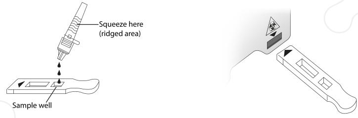
Test devices used in a laminar flow hood or in areas with high air flow should be covered during test development to ensure proper sample flow.
