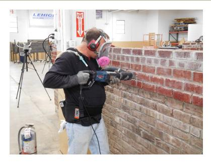
Figure 2 - Hammer drill with shroud and bit (NIOSH photo)
