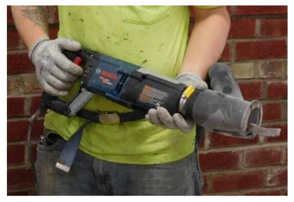
Figure 2 - Hammer drill with shroud and bit (NIOSH photo)
