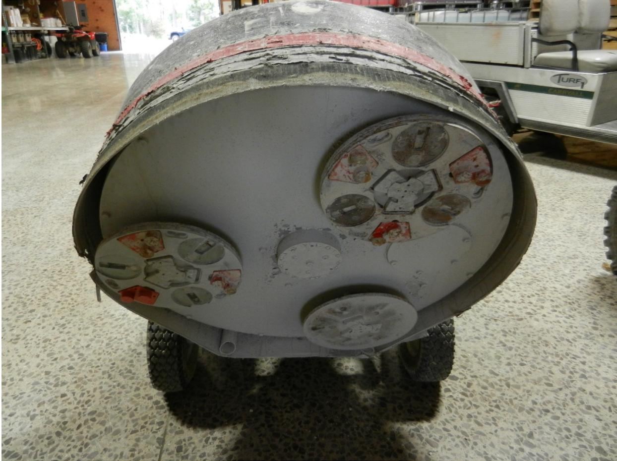
Figure 4: Shroud and polishing disks installed on the Concrete Polisher
