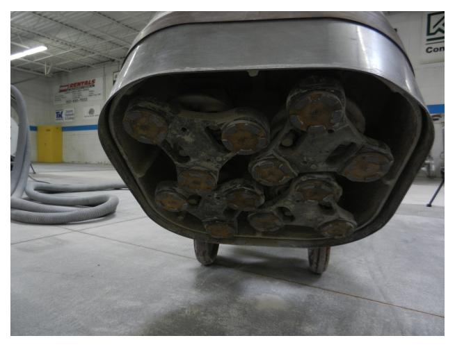
Figure 5: Shroud and polishing disks installed on the Concrete Polisher
