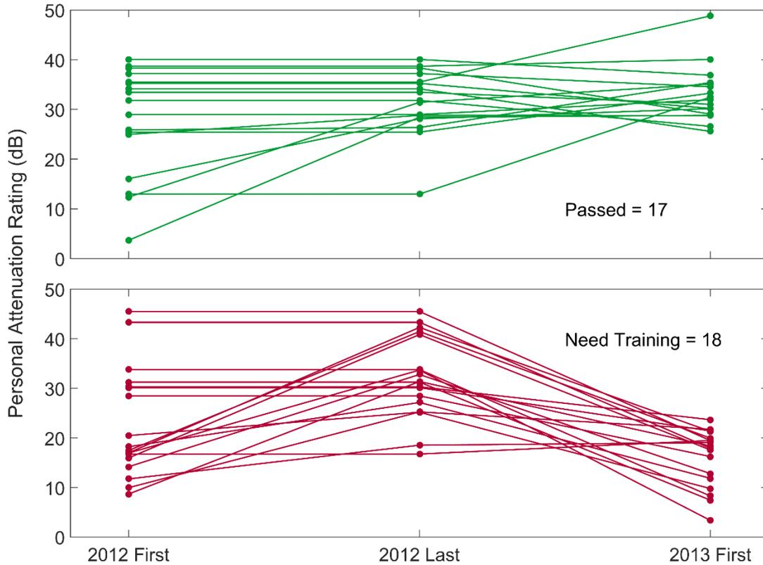
**Figure 9.** Fit test results over time for workers tested both in 2012 and 2013. Approximately half of the workers maintained the target 25 dB PAR between the final 2012 test and the initial 2013 test. Those who did not were retrained and illustrate the need to conduct fit-testing on a continual basis to ensure workers are properly protected.
