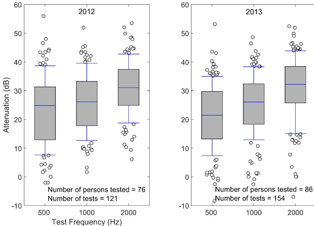
**Figure 8.** Fit-test results from the two field studies by frequency. The median, 25<sup>th</sup> and 75<sup>th</sup> quartiles are depicted with the box. The error bars indicate 5<sup>th</sup> and 95<sup>th</sup> percentiles. The data points outside the error bars have been shifted right and left with a random amount of jitter to facilitate visualization. The 2012 Louisiana attenuation data are displayed in the left panel and the 2013 Louisiana and Texas data are displayed in the right panel.
