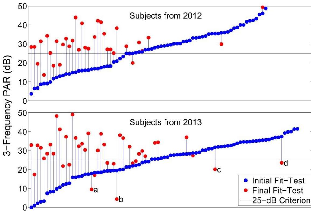
**Figure 7.** Initial and final personal attenuation ratings for BSEE workers in Louisiana and Texas fit-tested in 2012 (upper graph) and 2013 (lower graph). Results are sorted by ascending initial PARs. If only one result is shown, the worker was not re-tested. A few workers (points a-d) achieved lower PARs on their final fit-test than their initial fit-test; see text for details.
