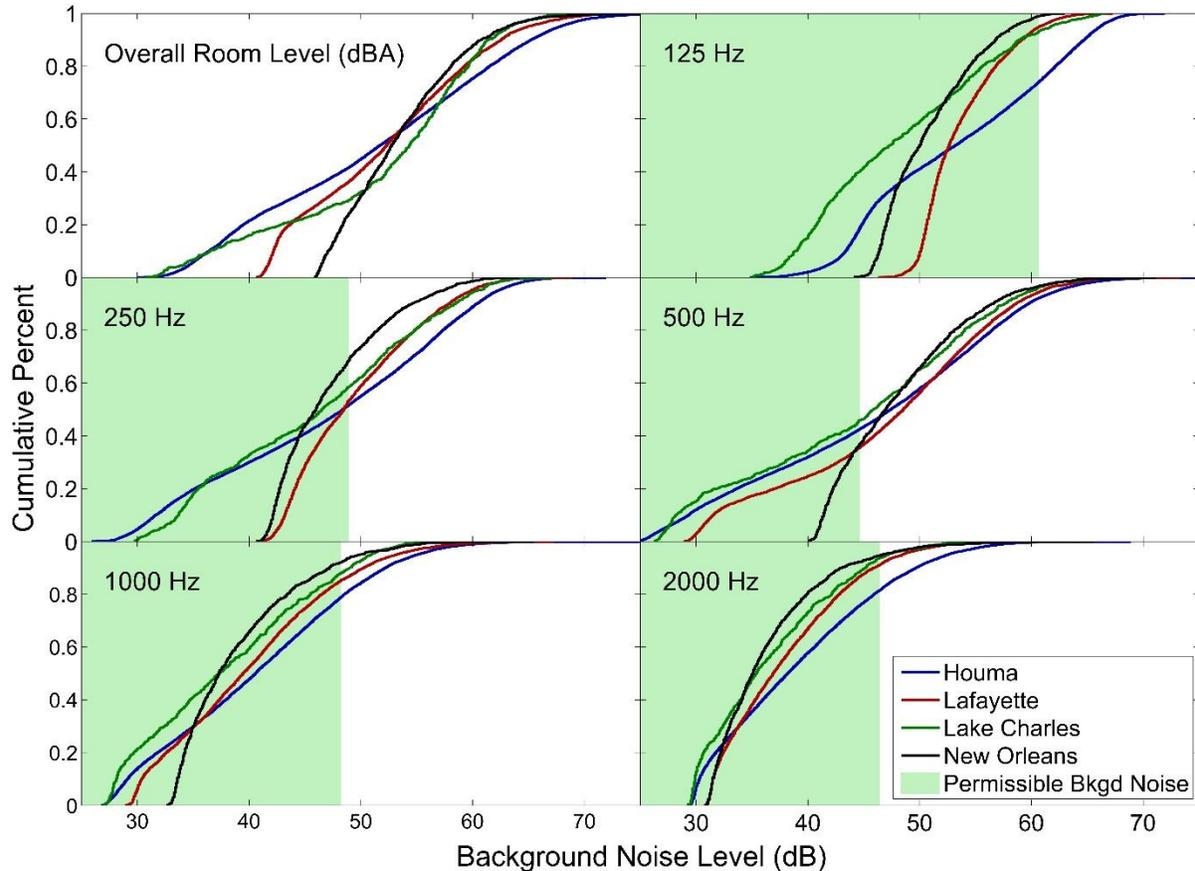
**Figure 11.** Cumulative distributions of overall and third-octave band ambient noise levels at each 2012 field survey site. The shaded area indicates the maximum level at which thresholds can be measured to audiometric zero, assuming a test range of 500 to 8000 Hz and taking into account the additional attenuation provided by the HPD Well-Fit headphones.
