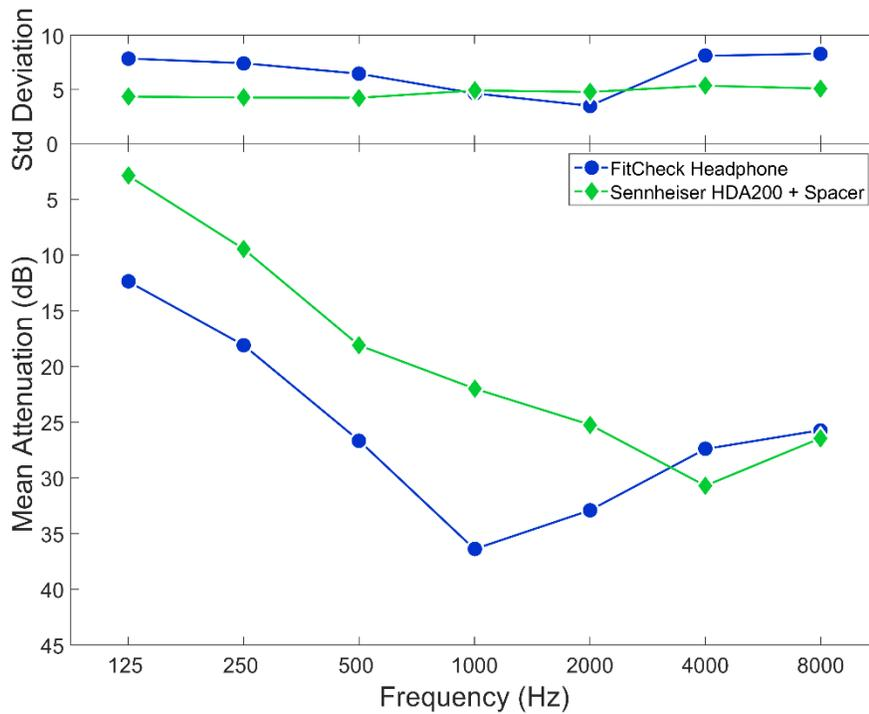
**Figure 5.** The attenuation as a function of frequency for the two circumaural headphones used with the HPD Well-Fit fit-test system. The attenuations for the Sennheiser HDA200 headphones at 500 to 2000 Hz provide at least 15 dB attenuation and the Michael & Associates FitCheck headphones provide at least 25 dB attenuation.
