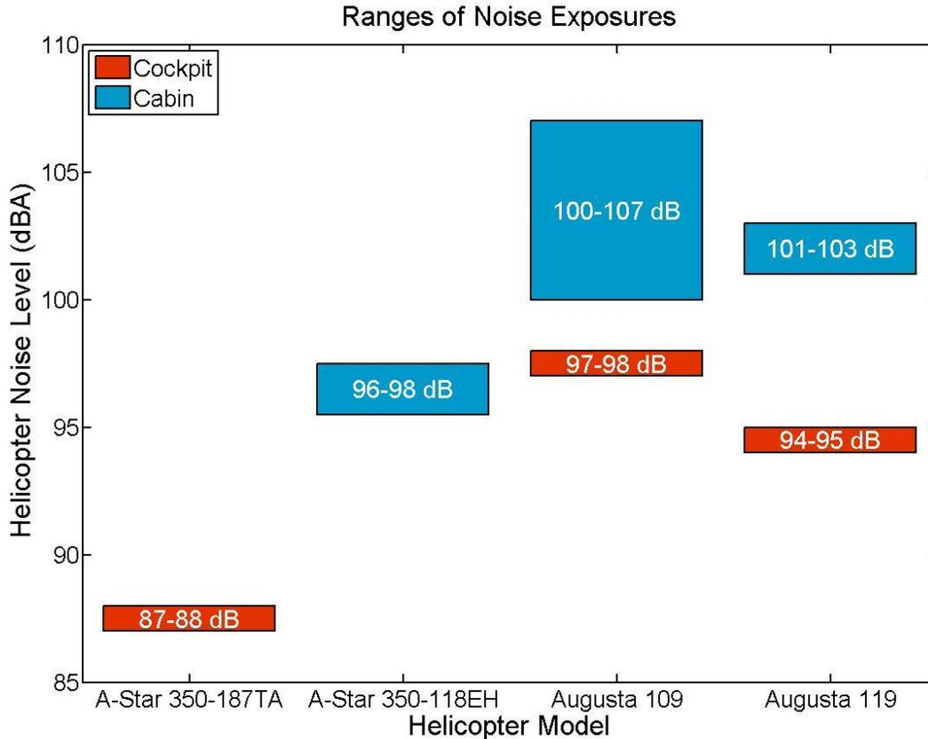
**Figure 2.** The range of noise exposure levels measured for four helicopters that were used to transport the workers. The orange bars illustrate levels measured in the cockpits of the helicopters while the blue bars are the levels measured in the cabins of the helicopters. Since the highest level was close to 110 dBA, a PAR value of 25 dB attenuation was chosen to protect the workers to 85 dBA.
