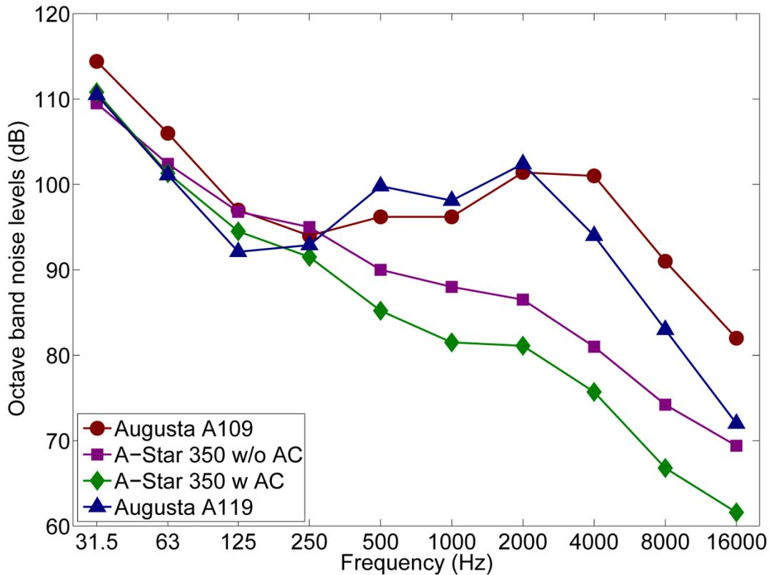
**Figure 3.** Octave band noise levels in dB SPL for helicopters commonly used to transport BSEE inspectors to off-shore oil rigs.
