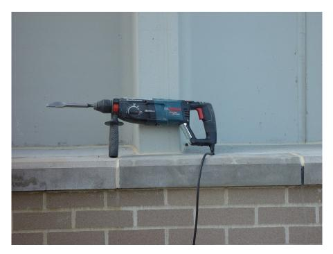
Figure 2 - Chisel Tool and Rotary Hammer (NIOSH photo)
