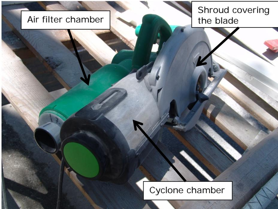
Figure 5 – The prototype red-spur saw with its built-in cyclone dust collector and air filter. Photo courtesy of NIOSH.
