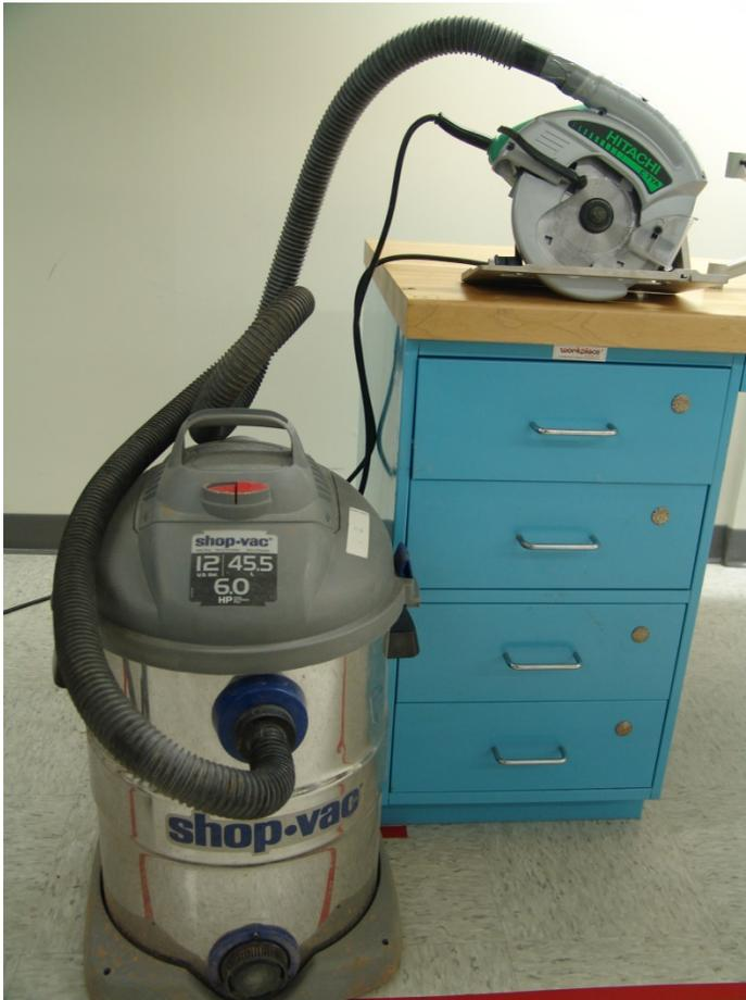
Figure 3 –The dust-collecting circular saw and its connection to the shop vacuum used in this survey.
